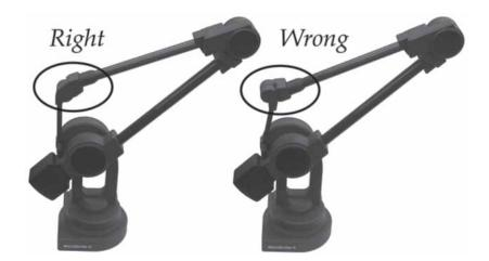
**Figure 1**. Correct and incorrect resting position (AKA Homing position) (Revware Systems 2009, MicroScribe G User Guide).
