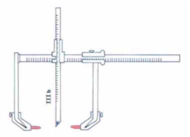
**Figure 9.** This is a radiometer (coordinate caliper) used for taking radii. The radiometer point is simulating the placement of the probes (in red) in the EAMs. Notice they are parallel and would "float" in the EAMs (Image from: Howells 1973, p. 164).
